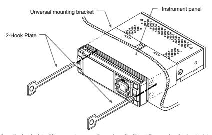
\* Keep the hook plate. You cannot remove the main unit without disengaging the hook plate.
